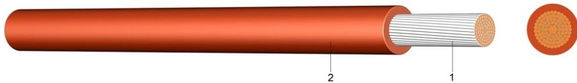
**Construction:** 1 ..... fine-stranded tinned copper
